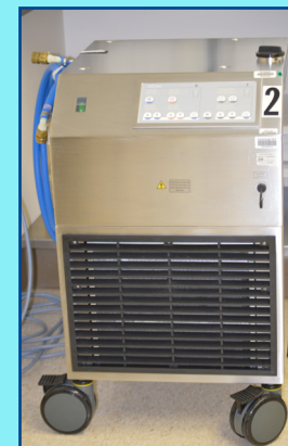
HCU is used to transfer heat or cold to the patient's blood in the bypass circuit to maintain a set body temperature
